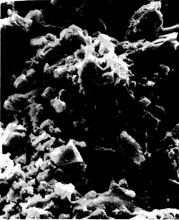
Figure 11 Micron Grain of Lunar Soil (1000 Magnification), Showing Agglutinate Composition
