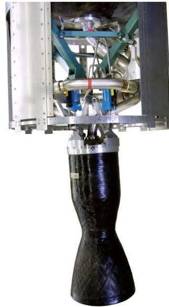
**Figure 9. 20K lbf Thrust Engine Apparatus.**
