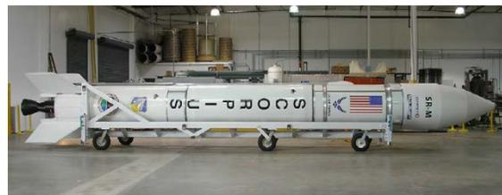
**Figure 13. SR-M Suborbital Launch Vehicle.**
