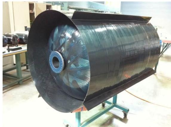
**Figure 5. All-Composite Tank with Skirts and Longitudinal Stringers.**
