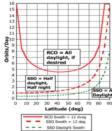
**Fig. 4. Single satellite orbits/day of coverage vs. latitude.**
