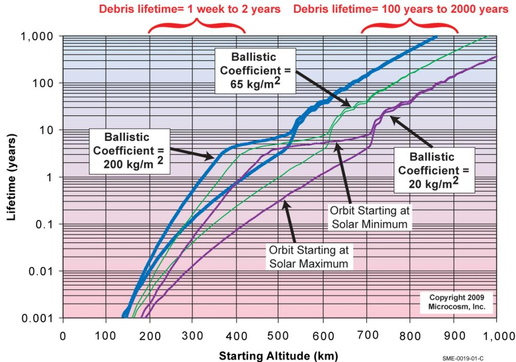
**Fig. 11. Satellite lifetime as a function of altitude. Operational SmallSats will typically inhabit a regime where orbital debris cannot accumulate.** (Underlying chart from Wertz [2009].)
