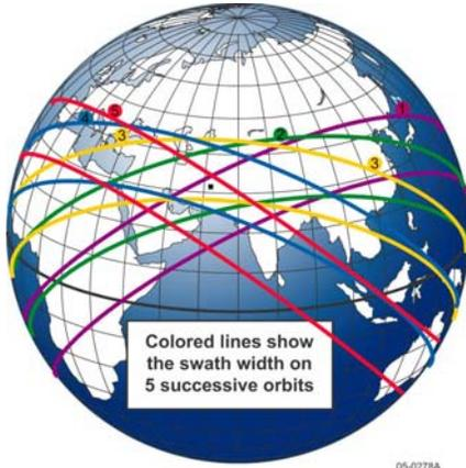
**Fig. 3. Repeat Coverage Orbit provides coverage of a particular region or latitude band on 4 to 6 successive orbits.**
