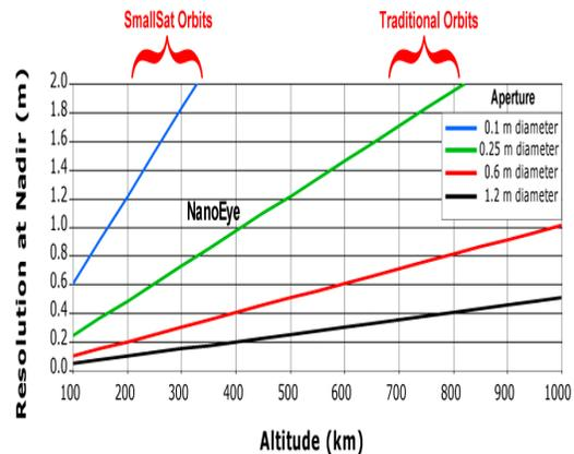
**Fig. 5. Resolution vs. Altitude for low altitude SmallSat orbits and higher altitude orbits used for more traditional systems.**
