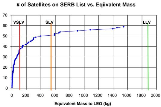
**Fig. 2. Satellites in the SERB list sorted by Equivalent Mass to LEO.** (Data compiled by Nicola Sarzi-Amade', Microcosm.)
