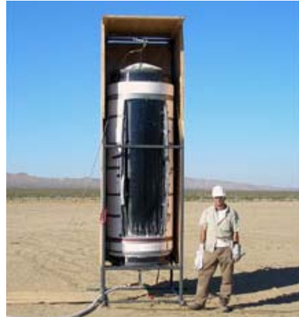
Figure 3. 42-in Diameter (Sprite) LOX Tank.
