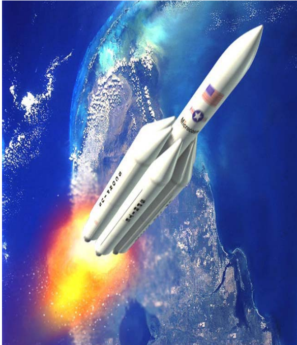
Figure 1. Pressure-fed Scorpius® Vehicle.
