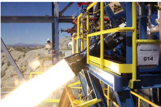
Figure 2. 20K lbf Engine Testing.
