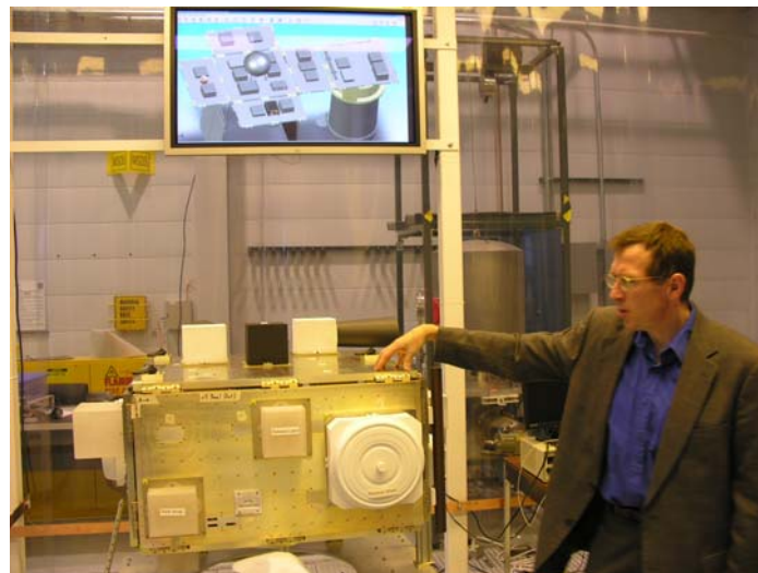
Fig. 8. "Concept bus", conceptual progenitor of the Plug-and-play Satellite
