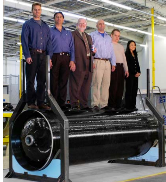
Figure 3. Composite Tank Strength Demo. Composite Tanks for Pressure-fed Launch Vehicles Display High Strength.
