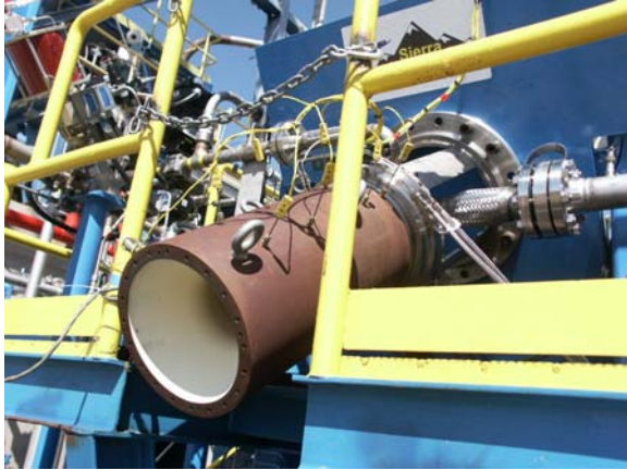
Figure 5: 20K lb f with Hardwall Chamber on Test Stand 2A at Edwards AFB.
