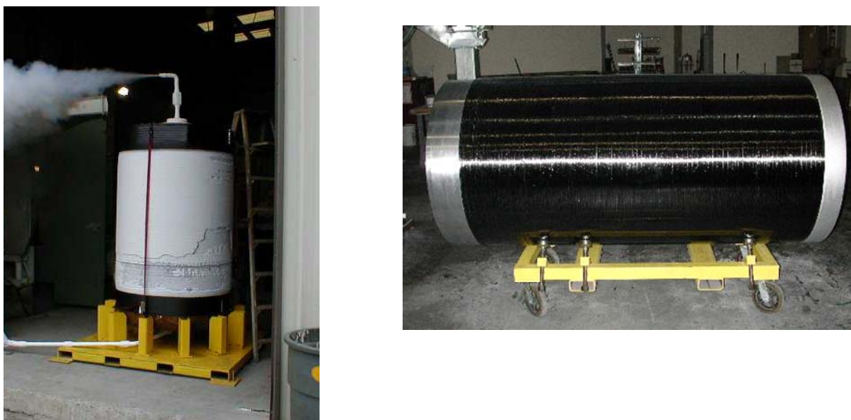
Figure 3: All-Composite LOX Tank (left) in Cryogenic Testing and Flight-Proven Fuel Tank (right).
