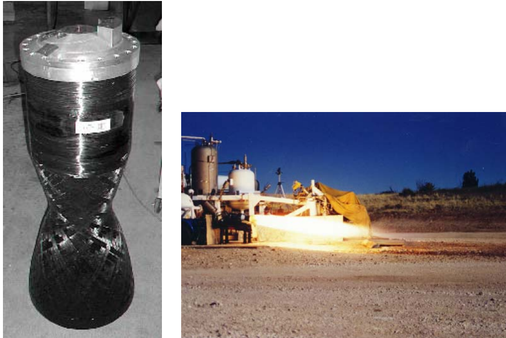
Figure 5: 20-klbf Ablative Engine (left) and 5-klbf Engine Hot Fire Testing (right).
