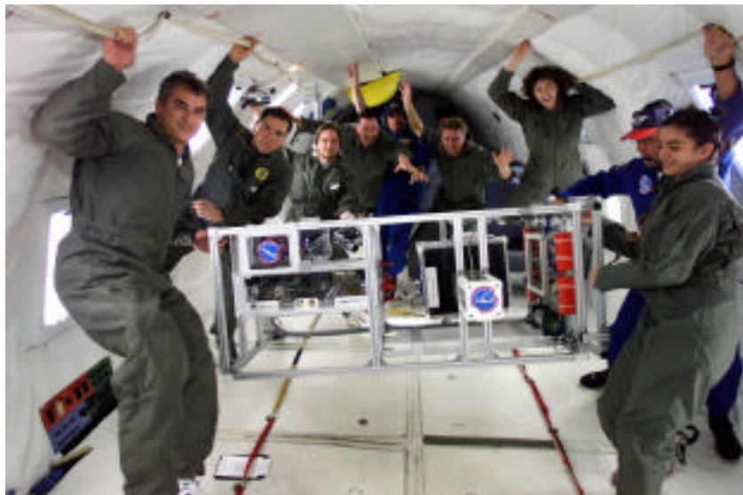
Figure 5. KC-135 Zero-Gravity Testing of a Small Spacecraft Docking Adapter Developed by Michigan.
