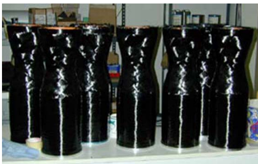
Figure 8. 5,000-lbf Thrust Chambers on the Left and 20,000-lbf Thrust Engine on the Right.
