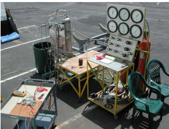
Figure 12. HPPS Based on Tridyne Technology in Testing at Microcosm.
