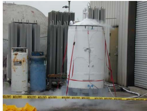
Figure 11. All-Composite LOX Tank During Cryo Testing.
