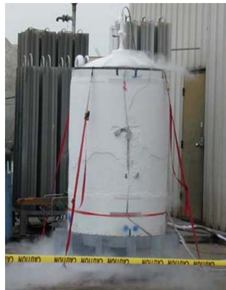
Figure 9. All-Composite LOX tank during development testing.
