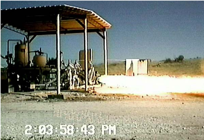
Figure 7. Typical Scorpius ® hardware, 20,000 lb. Engine firing and chamber.
