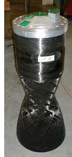
Figure 7. Typical Scorpius ® hardware, 20,000 lb. Engine firing and chamber.
