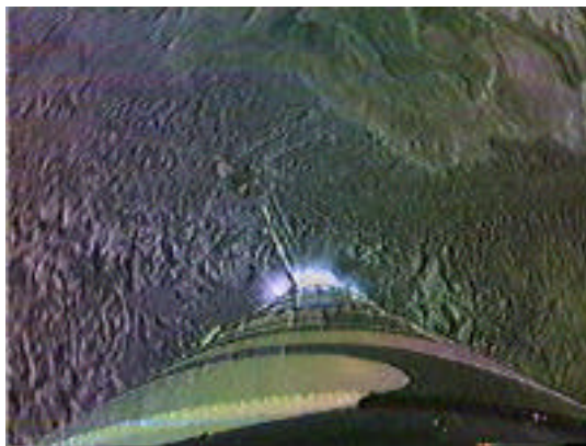
Figure 2. View from the SR-S Onboard Camera. The onboard camera provided real-time visual confirmation of the telemetry data, including the vehicle attitude motion. Onboard status information and GPS data were also telemetered back to verify the flight profile determined by the White Sands tracking network.
