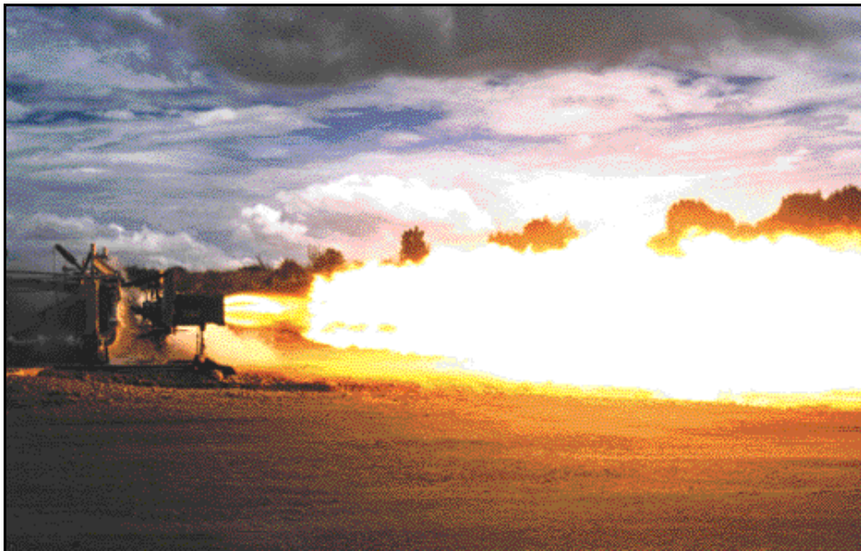
Figure 5. Testing of 40,000 lb. Thrust Engine at Socorro Test Site. These tests were used to characterize a 40,000 lb. thrust injector developed by TRW for the Scorpius program.
