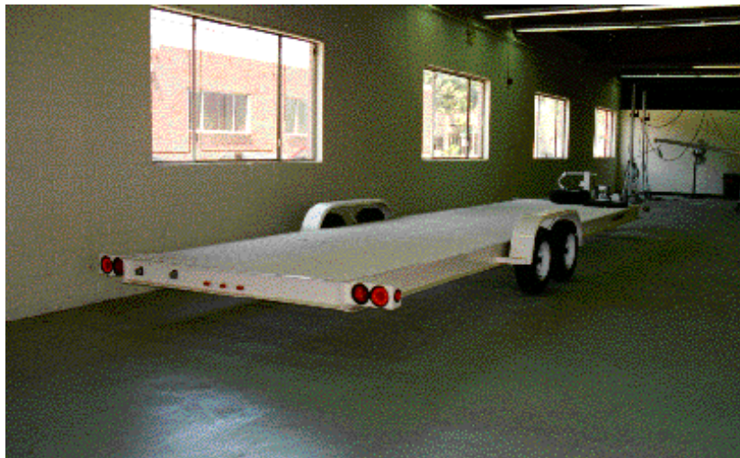
Fig. 4. The Scorpius Integration Facility. Showing the transport trailer for both the SR-S and SR-1 suborbital vehicles. Vehicle specific adapters (not shown) will allow either vehicle to be transported and erected.
