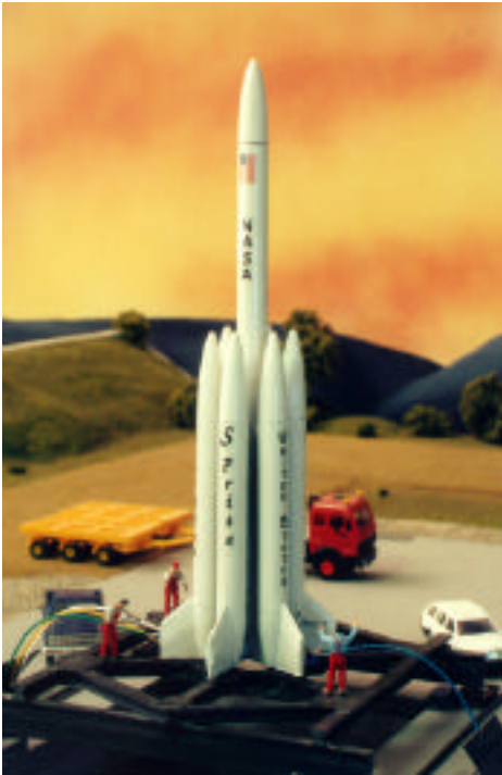
Fig. 2. The Sprite Mini-lift Launch Vehicle. Sprite was intended to put 330 lbs into low Earth orbit at a recurring cost of $1.5 million by the middle of calendar year 2000.
