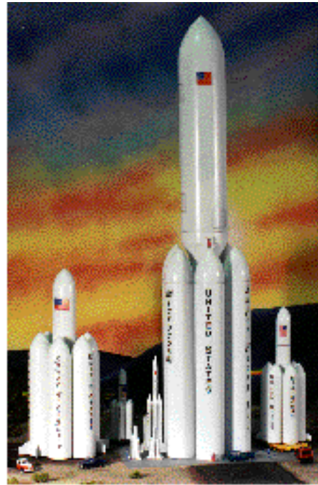
Fig. 3. The New Scorpius Vehicle Family. Suborbital vehicles in the foreground. Background from left: Heavy Lift, Liberty Light Lift, Sprite Mini-lift, Super Heavy Lift, Exodus Medium Lift.
