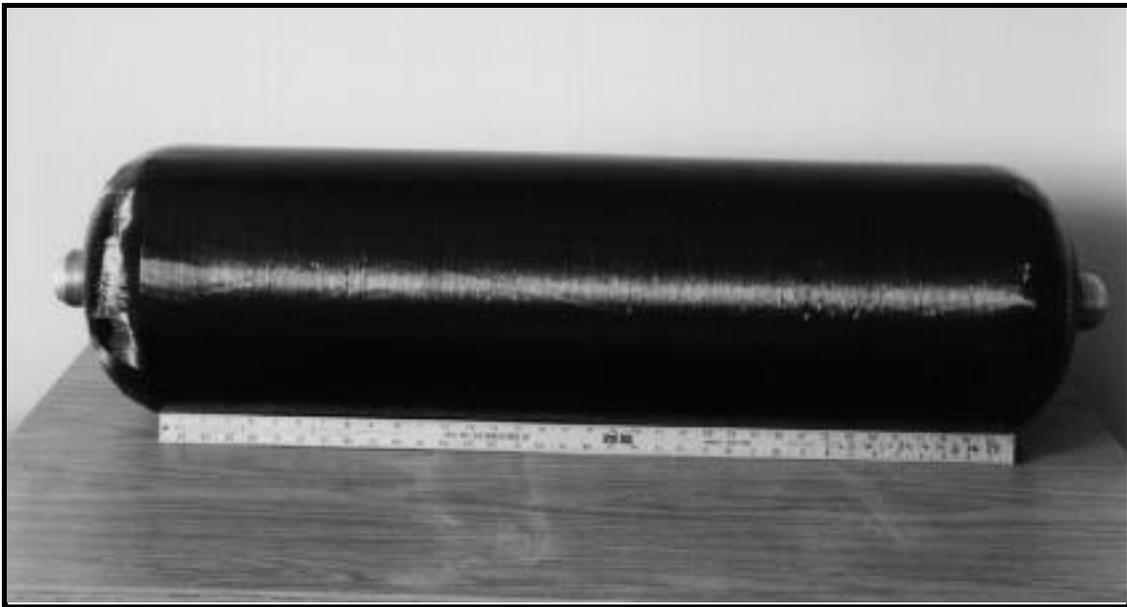
**Figure 6. *Scorpius* test tanks.** The tanks have a metallic liner and will be tested shortly for performance in holding LOX and kerosene.
