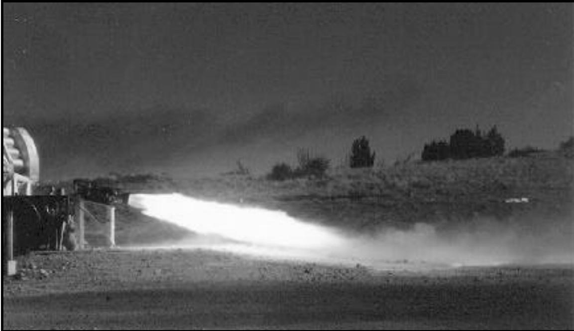
**Figure 4. 200 sec *Scorpius* engine test at RTF on Nov. 18, 1995.** All performance parameters were nominal. Achieved engine life exceeded requirements for launch to orbit with substantial life left on the engine.
