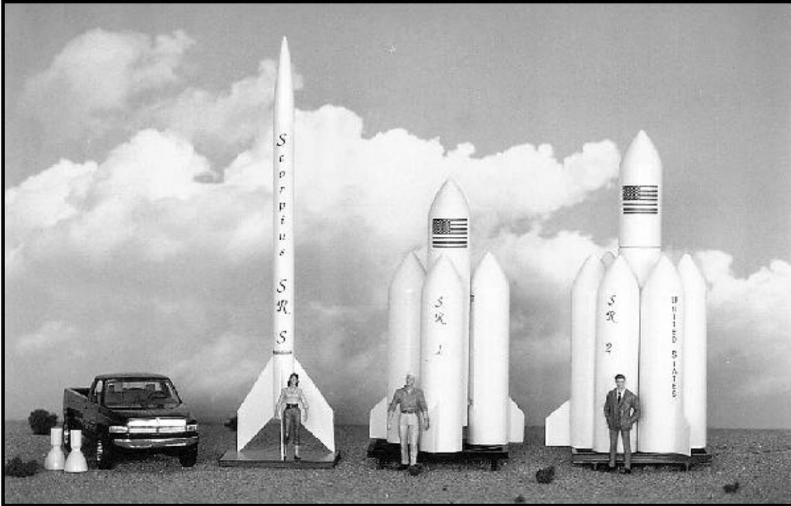
**Figure 3. The *Scorpius* Suborbital Rocket Family.** From left the vehicles are the SR-S single-stage rocket, the SR-1, 3-engine, single-stage vehicle, and the SR-2, two-stage vehicle.
